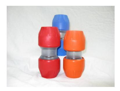
The Clear-Loc coupling is designed for easy application and allows quick installation in all types of situations, especially where tight installation conditions exist. The coupling is designed without a center stop, and the clear body allows for visual verification that the innerducts are centered and properly aligned. It is airtight and will hold air pressures of 150psi when installed properly.
